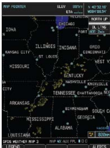
Figure 4-111 GFDS Data Link Lightning and Legend
